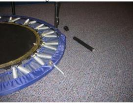
Step 4: Using the Cotter Pin Tool or other similar tools (a small screwdriver, hammer, and pliers), remove the cotter pin from the leg base. This will allow the spring to release. Discard old spring.
