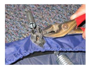
Step 5: Place new spring into the leg base and reattach at the coiled end lightly tap the pin back through leg base with a hammer or similar tool until the cotter pin is back in place.
